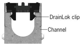
ACO **DrainLok™** is a patented, boltless locking system that removes the need for bolts and bars and improves the hydraulic capacity of the channel. The **DrainLok™** mechanism simply clips into the channel edge rail for rapid installation. ACO **DrainLok™** grates are fitted with an anti-shunt mechanism that restricts unwanted grate movement when installed, improving durability and longevity of the system.
